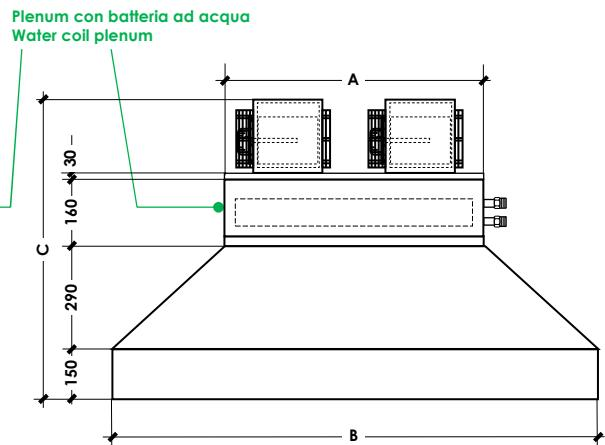
**BARRIERE CON BATTERIA AD ACQUA**
