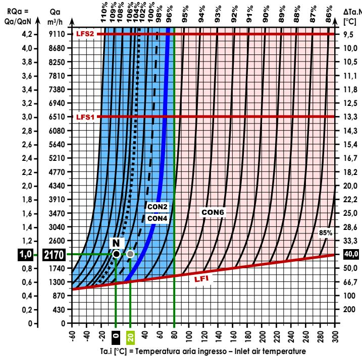
**22 kW (80% Pn)** $\eta$  % (@Hi, Metano/Methane G20 (100%CH4), Ta.c20°C, 10%CO2)
